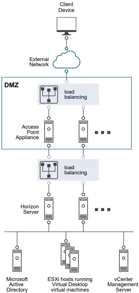
Alternatively you can have one or more Access Point appliances pointing to an individual server instance. In both approaches, use a load balancer in front of two or more Access Point appliances in the DMZ.
