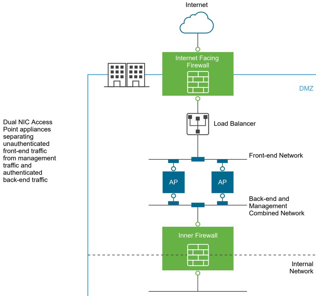
In a two NIC deployment, traffic going to the internal network through the inner firewall must be authorized by Access Point. Unauthorized traffic is not on this back-end network. Management traffic such as the REST API for Access Point is only on this second network
