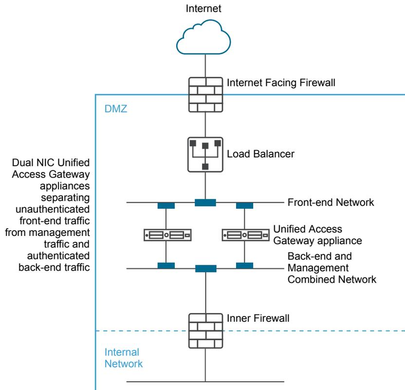
In a two NIC deployment, Unified Access Gateway must authorize the traffic going to the internal network through the inner firewall. Unauthorized traffic is not on this back-end network. Management traffic such as the REST API for Unified Access Gateway is only on this second network
