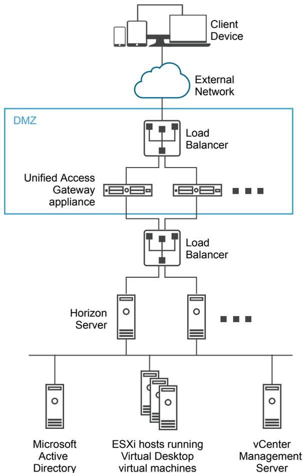
Alternatively you can have one or more Unified Access Gateway appliances pointing to an individual server instance. In both approaches, use a load balancer in front of two or more Unified Access Gateway appliances in the DMZ.
