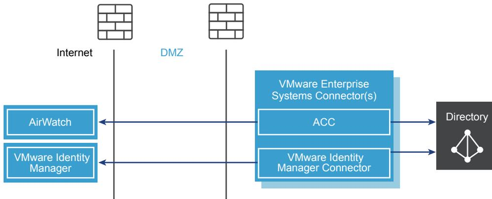
The following diagram shows the deployment of the ACC component only.
