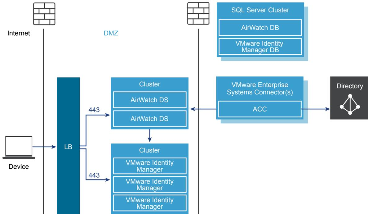
The following diagram shows the deployment of both the ACC and VMware Identity Manager Connector components with a typical on-premises AirWatch layout.
