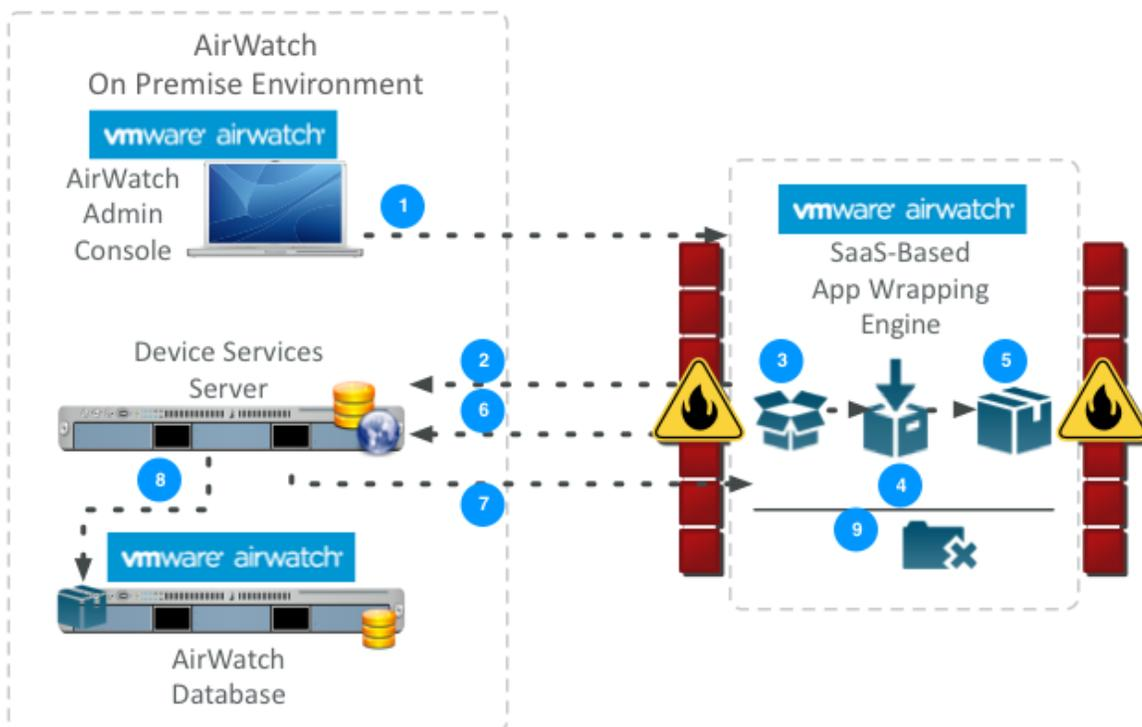
1. The admin uploads the internal application and ancillary files, like provisioning profiles and signing certificates, to the AirWatch Console and initiates wrapping.
