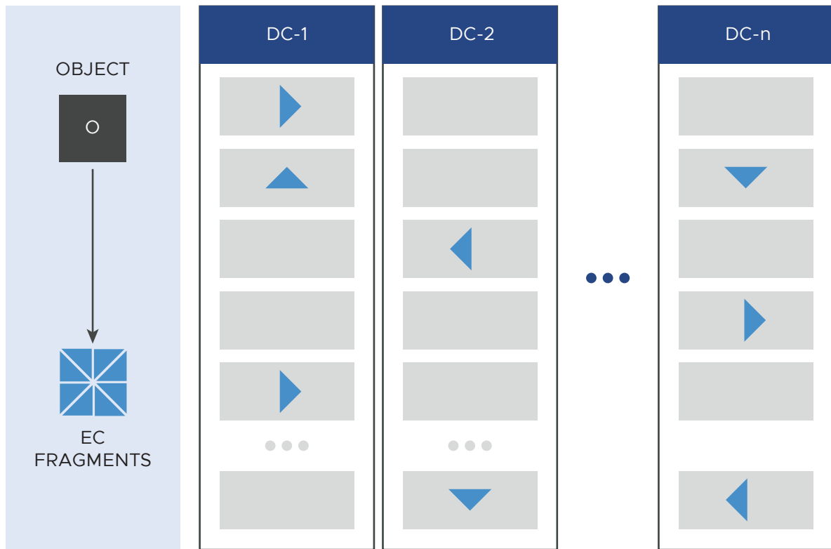
Figure 9-3. Erasure coding across data centers
