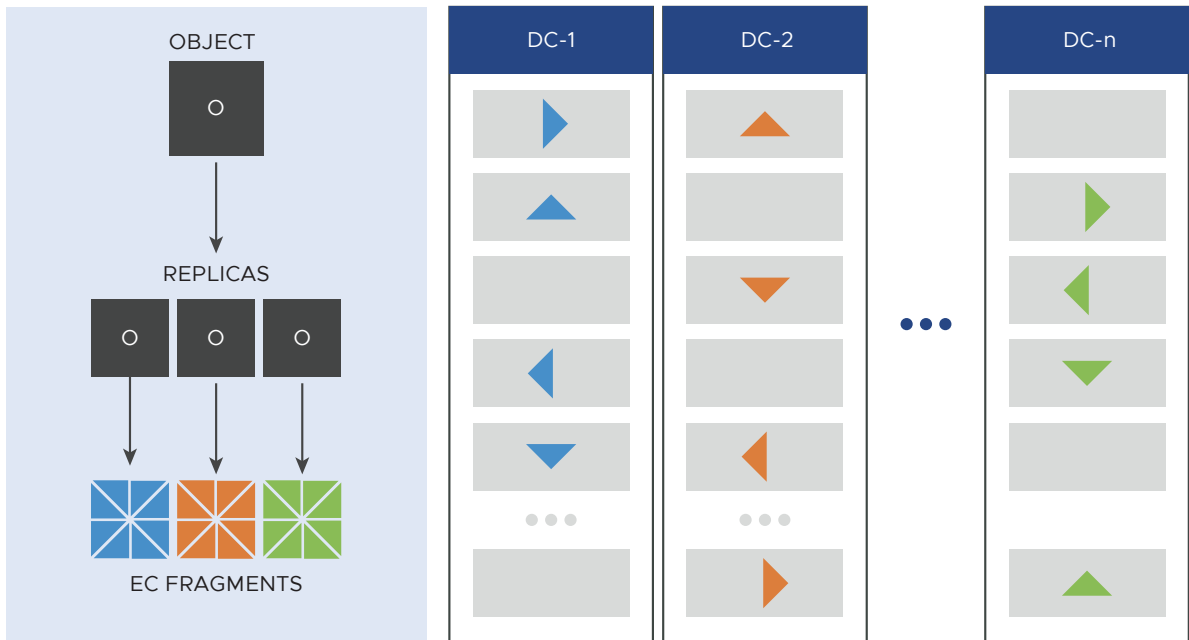
Figure 9-5. Replicated erasure coding across multiple data centers
