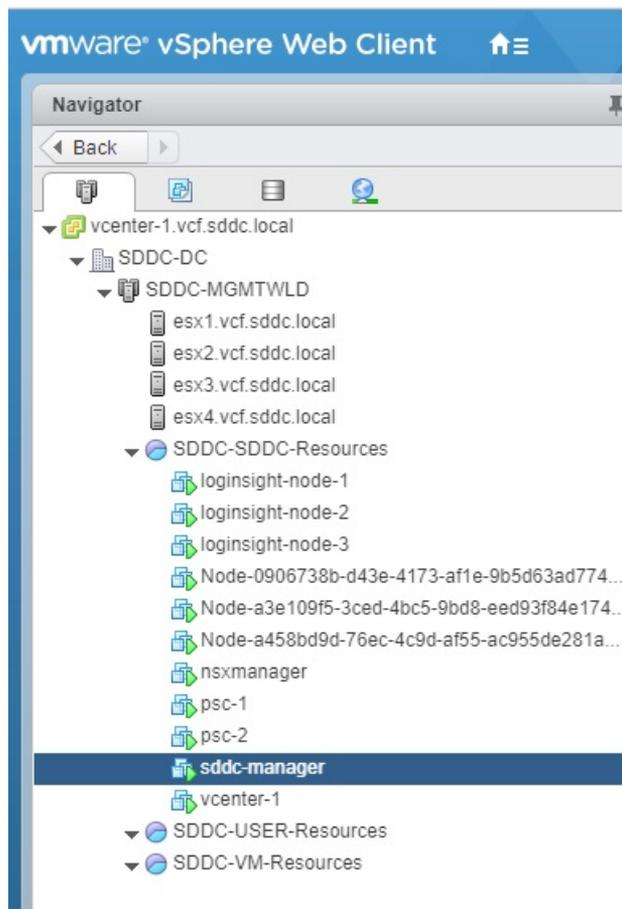
Within this cluster are a series of virtual machines that have been automatically deployed by Cloud Foundation. These include:
