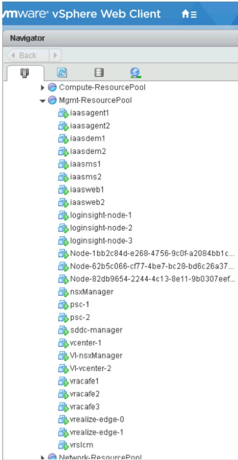
In addition, vRealize Automation has been deployed. Deploying vRealize Automation is optional. A vRealize Life Cycle Management (VRLCM) appliance and NSX edge devices are deployed for vRealize Automation. These components are shared with vRealize Operations and are only deployed once, even if you deploy both vRealize Operations Manager and vRealize Automation.
