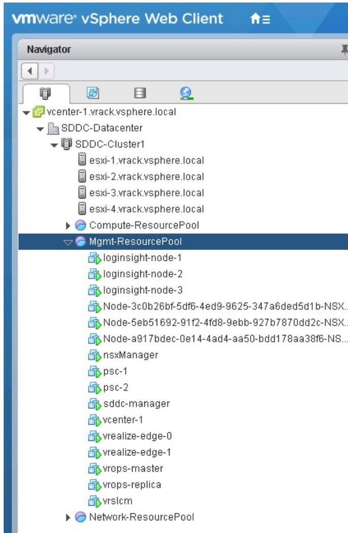
The deployment of vRealize Operations Manager within the environment is optional. In this example, vRealize Operations Manager was deployed with two nodes. You can define the number of nodes to be deployed as part of vRealize Operations Manager. See the *VMware Cloud Foundation Operations and Administration Guide* for more information on deploying vRealize Operations Manager within Cloud Foundation.
