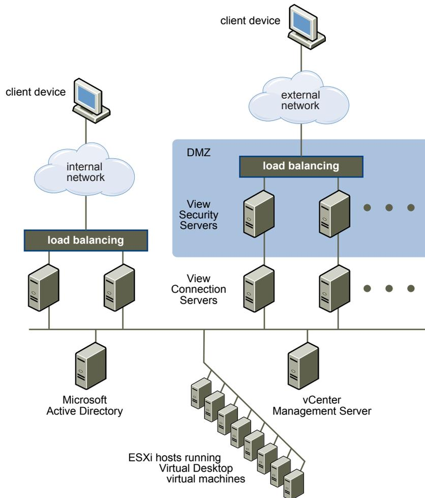
You must implement a hardware or software load balancing solution if you install more than one security server. View Connection Server does not provide its own load balancing functionality. View Connection Server works with standard third-party load balancing solutions.
