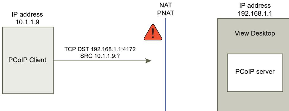
To resolve this problem, you must configure the plug-in to use an external IP address. If `externalIPAddress` is configured as 10.1.1.1 for this desktop, the plug-in gives the client an IP address of 10.1.1.1 when making desktop protocol connections to the desktop. For PCoIP, the PCoIP Secure Gateway service must be started on the desktop for this setup.
