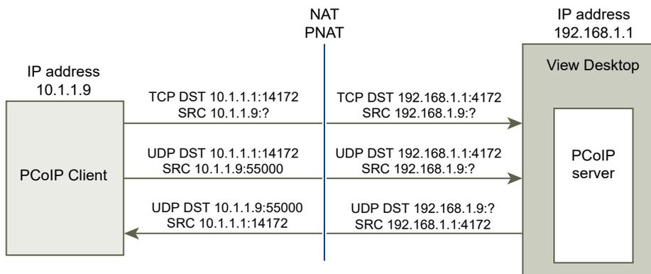
As with the external PCoIP TCP/UDP port configuration for PCoIP, if the RDP port (3389) or the Framework Channel port (32111) is port mapped, you must configure `externalRDPPort` and `externalFrameworkChannelPort` to specify the TCP port numbers that the client will use to make these connections through a port mapping device.
