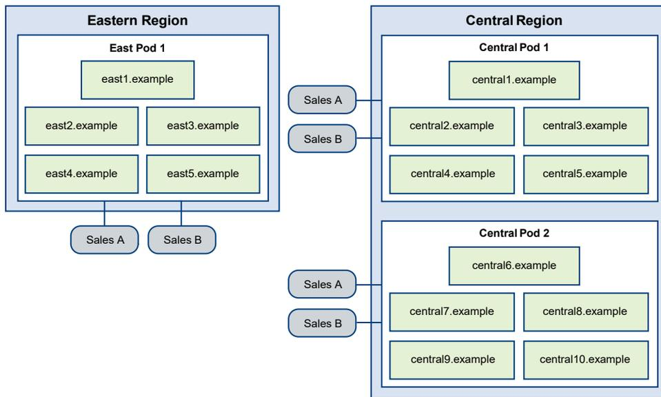
In this topology, the Eastern region site contains a single pod, East Pod 1, that consists of five Connection Server instances called east1.example through east5.example.
