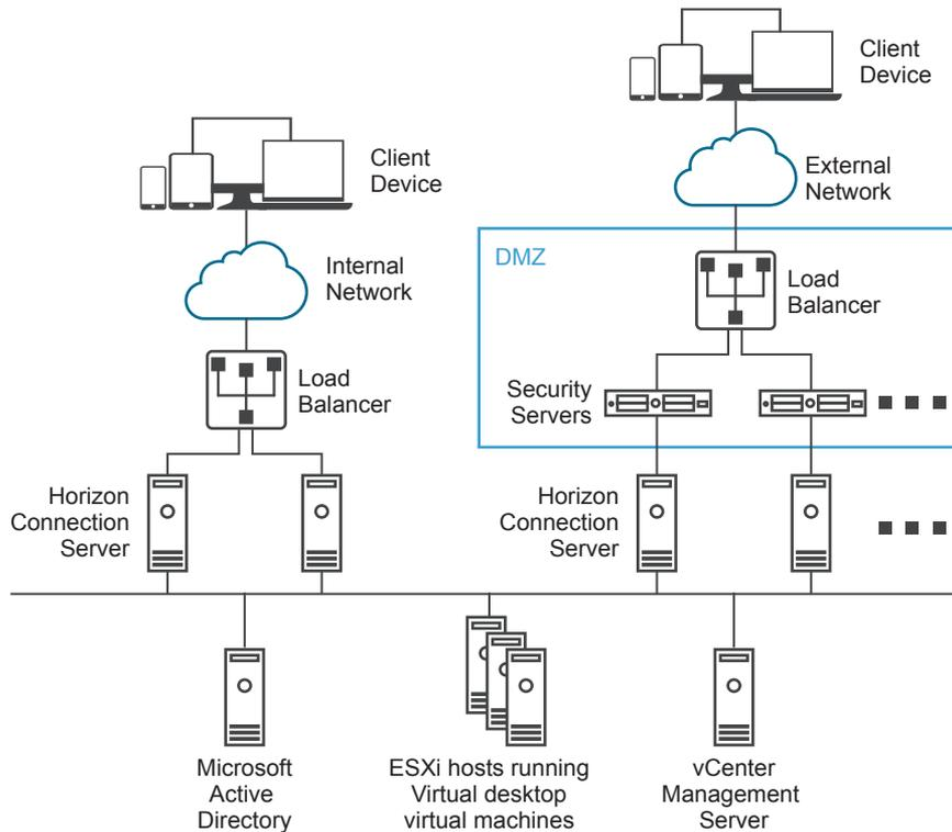
You must implement a hardware or software load balancing solution if you install more than one security server. Connection Server does not provide its own load balancing functionality. Connection Server works with standard third-party load balancing solutions.
