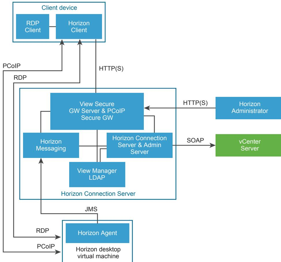
**Note** This figure shows direct connections for clients using either PCoIP or RDP. The default setting, however, is to have direct connections for PCoIP and tunnel connections for RDP.
