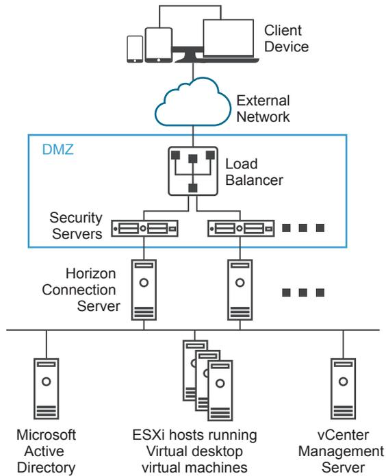
When users outside the corporate network connect to a security server, they must successfully authenticate before they can access remote desktops and applications. With appropriate firewall rules on both sides of the DMZ, this topology is suitable for accessing remote desktops and applications from client devices located on the Internet.
