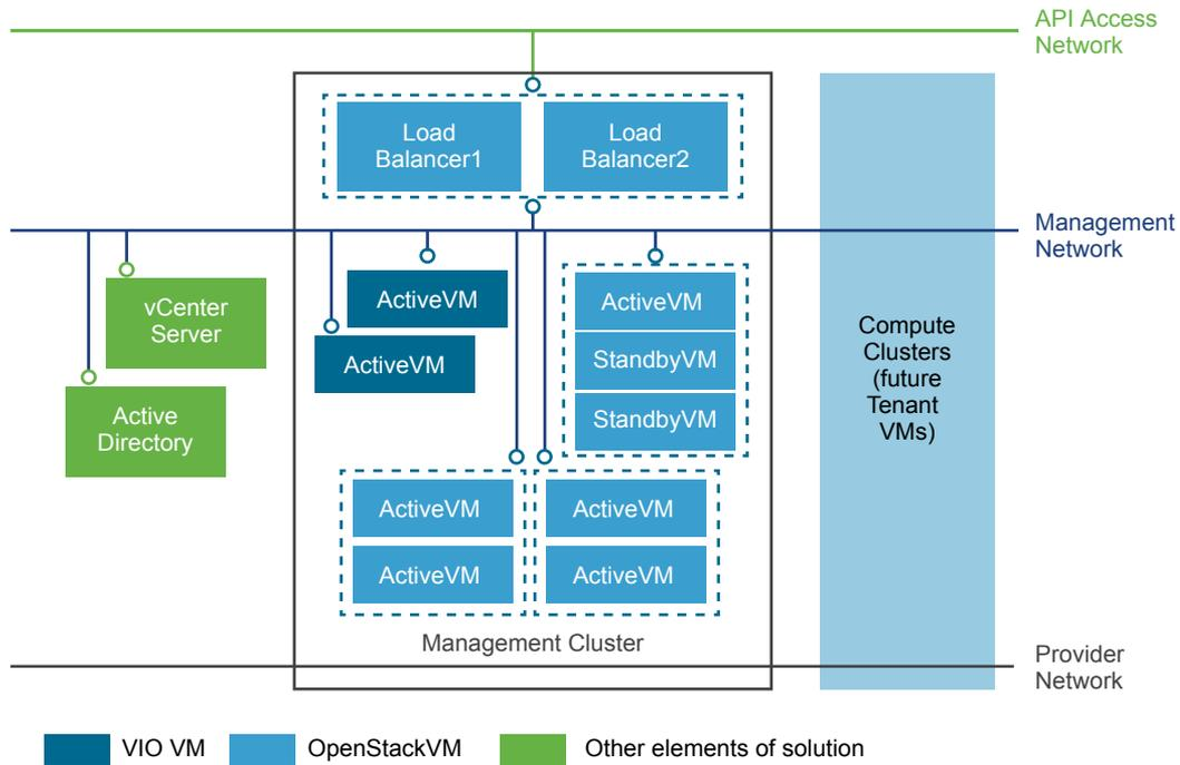
The VMware Integrated OpenStack architecture includes the following clusters and components.
