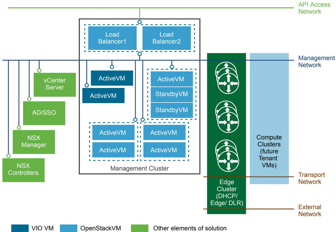
The VMware Integrated OpenStack architecture includes the following clusters and components.
