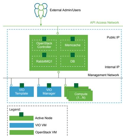
If you are comfortable protecting the virtual machine by making regular backups, then you can use compact architecture in production. If you are not comfortable making regular backups, the compact architecture is good for learning, proof of concept, and evaluating new versions of VIO.
