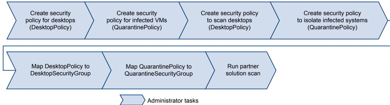
**Figure 17-7. Service Composer Conditional Workflow**
