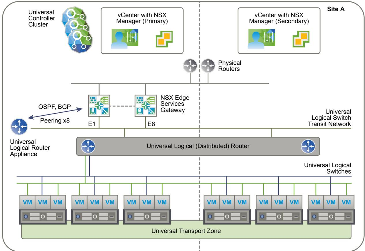
Figure 4-2. Cross-vCenter NSX spanning two sites
