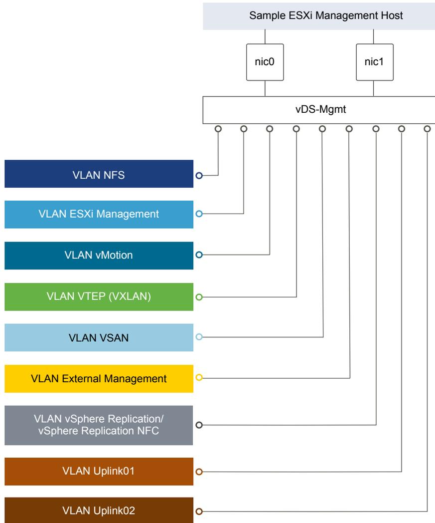
This section expands on the logical network design by providing details on the physical NIC layout and physical network attributes.
