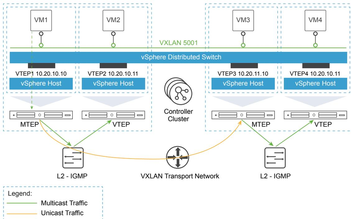
This design uses hybrid mode for control plane replication.
