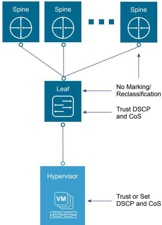
Two types of QoS configuration are supported in the physical switching infrastructure.
