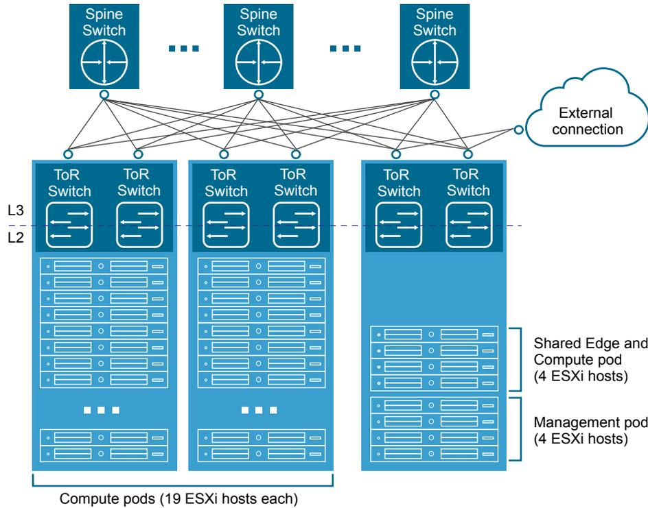
The number of links to the spine switches dictates how many paths for traffic from this rack to another rack are available. Because the number of hops between any two racks is consistent, the architecture can utilize equal-cost multipathing (ECMP). Assuming traffic sourced by the servers carries a TCP or UDP header, traffic distribution can occur on a per-flow basis.
