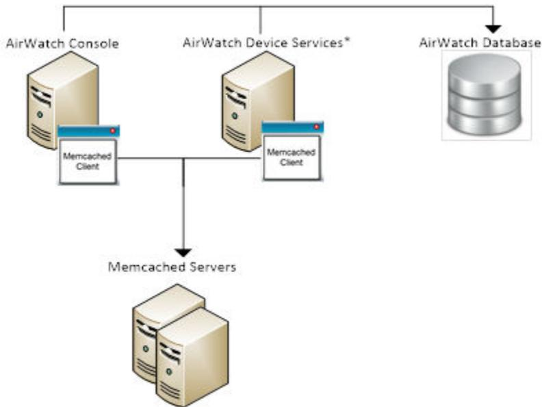
This diagram assumes that all auxiliary components – for example, API or SSP – are installed on the Device Services server. If you have dedicated servers for these or other components that have access to the AirWatch database, map those servers into your Memcached network topology.
