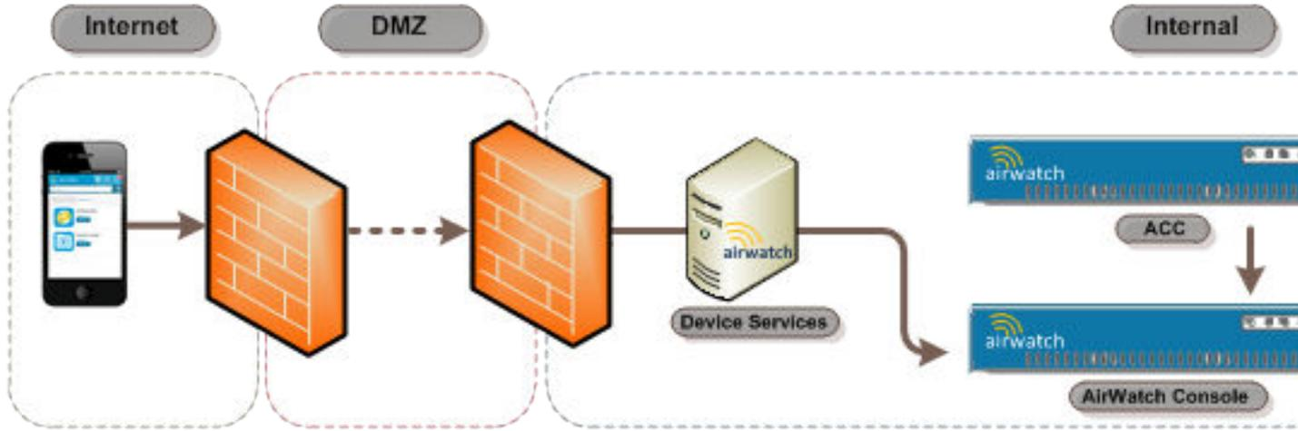
**Scenario #4 – On Premise: Device Services is located in the DMZ. VMware Enterprise Systems Connector, Workspace ONE UEM servers, and CA are internal.**
