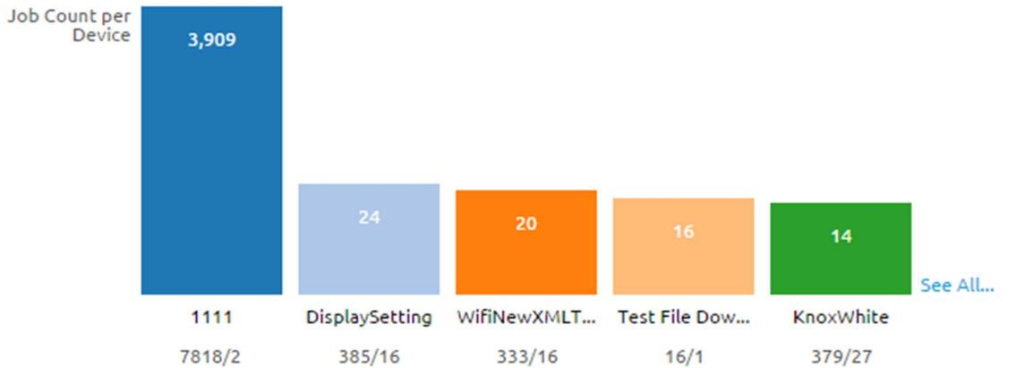
For example, if the number shown is a 3, then you know that an average of 3 jobs per device happens for this product. If you select the bar for each product, the View Devices screen displays with all devices currently assigned the product. You can then determine which jobs are failing and the reason for those failures.
