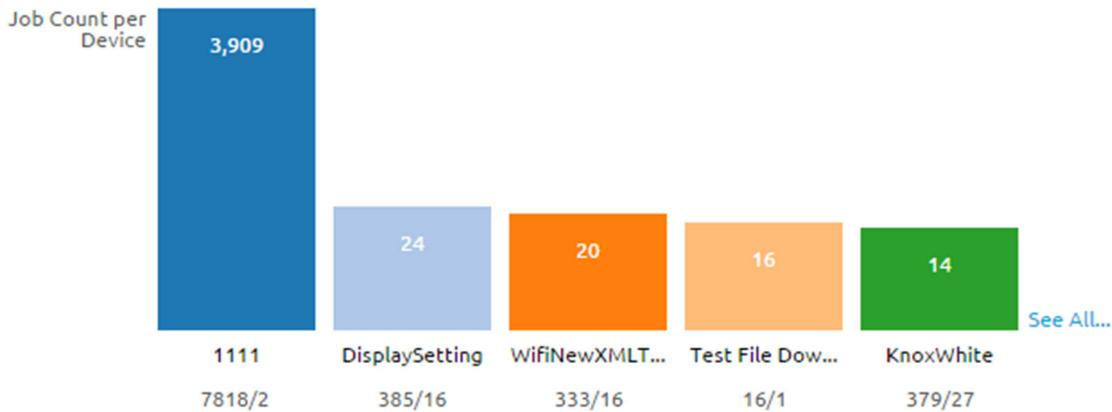
For example, if the number shown is a 3, then you know that an average of 3 jobs per device happens for this product. If you select the bar for each product, the View Devices screen displays with all devices currently assigned the product. You can then determine which jobs are failing and the reason for those failures.
