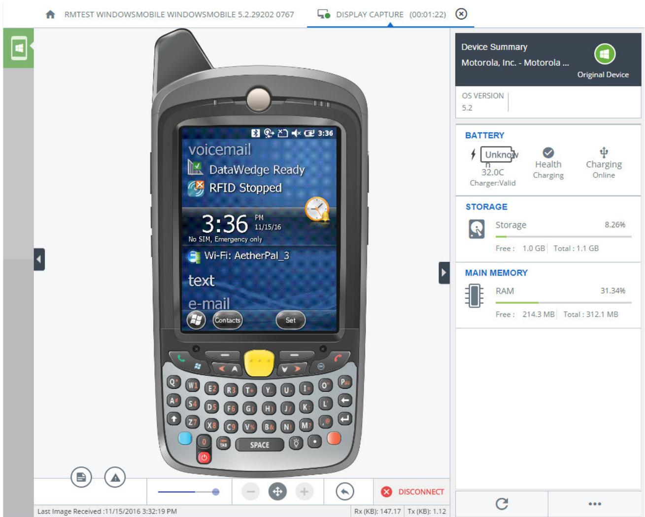
Control the device by clicking or dragging on the displayed screen and buttons. You can send keystrokes to the device and copy and paste information onto the device during a session.
