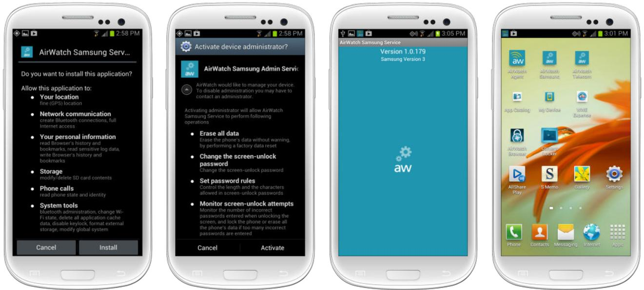
After installing the Workspace ONE Intelligent Hub, you are automatically prompted to begin installing the service app. Select **Install**, when prompted.
