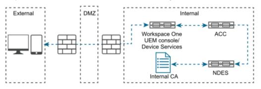
If you do not want to expose your SCEP endpoints to external devices, you can use the SCEP Proxy. This feature, **Enable Proxy**, is an advanced feature when you configure the CA in the Workspace ONE UEM console. The SCEP Proxy allows Workspace ONE UEM to act as an intermediary between the SCEP server and the device. It forwards and returns requests and responses between the two components. Workspace ONE UEM does not have the SCEP server's private key, so it cannot parse requests from devices.
