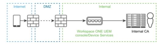
On-Premises - Devices Services in a DMZ with no VMware AirWatch Cloud Connector - In an onpremises environment, Devices Services is located in a DMZ and the CA and Workspace ONE UEM servers are internal. The VMware AirWatch Cloud Connector is not installed.
