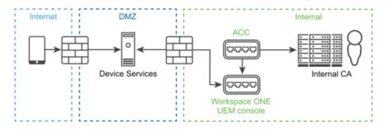
SaaS – Components in the Cloud with VMware AirWatch Cloud Connector - In a SaaS environment, Devices Services, Workspace ONE UEM server, and the CA are in the clou4. The VMware AirWatch Cloud Connector and an internal CA are internal and must be in the same domain.
