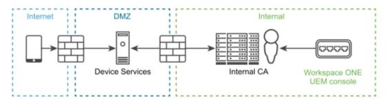
On-Premises – Components are Internal with VMware AirWatch Cloud Connector - In an onpremises environment, Devices Services, Workspace ONE UEM server, the CA, and VMware AirWatch Cloud Connector are internal.
