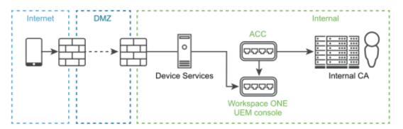
On Premises - Device Services in a DMZ with VMware AirWatch Cloud Connector - In an onpremises environment, Devices Services is located in the DMZ and Workspace ONE UEM server, CA, and VMware AirWatch Cloud Connector are internal.
