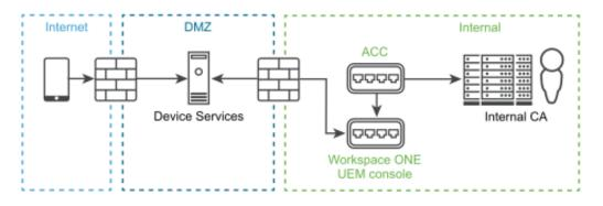
SaaS - Workspace ONE UEM as SaaS. AirWatch Cloud Connector and CA are internal. The ACC and CA must be in the same domain.
