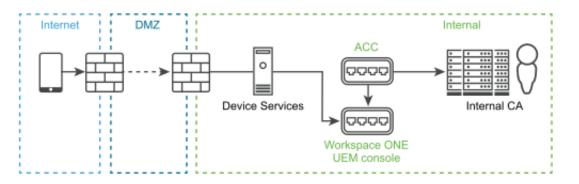
On Premises - Device Services is located in the DMZ. AirWatch Cloud Connector, Workspace ONE UEM servers, and CA are internal.
