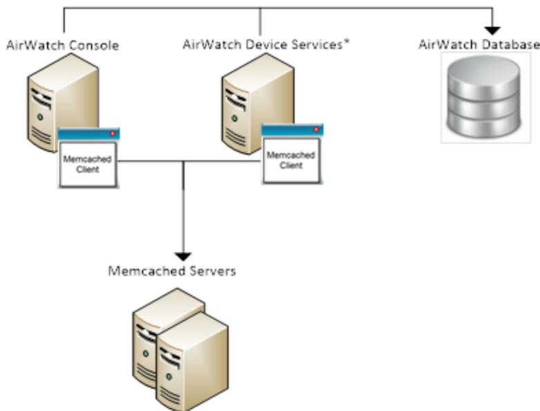
This diagram assumes that all auxiliary components – for example, API or SSP – are installed on the Device Services server. If you have dedicated servers for these or other components that have access to the AirWatch database, map those servers into your Memcached network topology.
