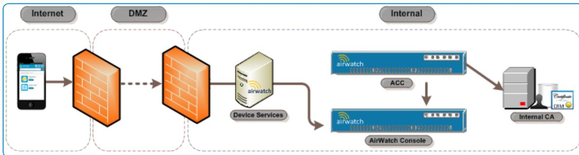
**Scenario #4 – On Premise: Device Services is located in the DMZ. VMware Enterprise Systems Connector, Workspace ONE UEM servers, and CA are internal.**
