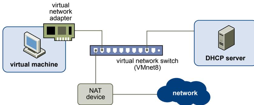
The virtual machine and the host system share a single network identity that is not visible on the external network. NAT works by translating the IP addresses of virtual machines in the private network to the IP address of the host system. When a virtual machine sends a request to access a network resource, it appears to the network resource as if the request is coming from the host system.
