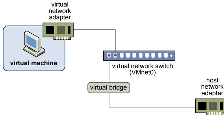
You can view and change the settings for bridged networking on the host system, determine which network adapters to use for bridged networking, and map specific host network adapters to specific virtual switches.
