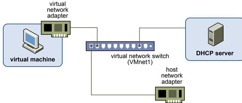
In the default configuration, a virtual machine in a host-only network cannot connect to the Internet. If you install the proper routing or proxy software on the host system, you can establish a connection between the host virtual network adapter and a physical network adapter on the host system to connect the virtual machine to a Token Ring or other non-Ethernet network.
