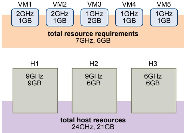
The total resource requirements for the powered-on virtual machines is 7GHz and 6GB. The total host resources available for virtual machines is 24GHz and 21GB. Based on this, the Current CPU Failover Capacity is 70%  $((24\text{GHz} - 7\text{GHz})/24\text{GHz})$ . Similarly, the Current Memory Failover Capacity is 71%  $((21\text{GB} - 6\text{GB})/21\text{GB})$ .
