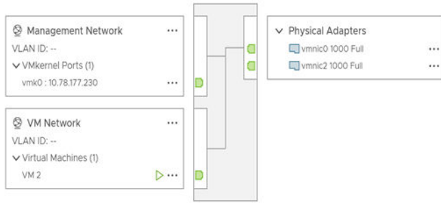
Figure 2-2. Topology Diagram of a vSphere Standard Switch
