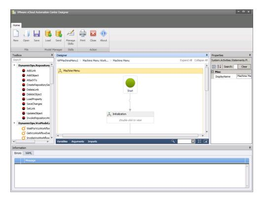
The Toolbox pane on the left provides access to the vRealize Automation workflow activity library. You can drag activities from the toolbox onto the Designer pane to add them to a workflow. The Properties pane displays the configurable properties of the currently selected activity on the Designer pane. This interface is very similar to the workflow designer in Visual Studio.
