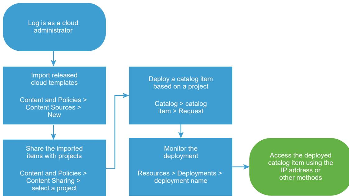
In this use case, you import released Cloud Assembly cloud templates. You can also import Amazon CloudFormation templates, but the process is not presented here. See [Add CloudFormation Templates to the Service Broker Catalog](#) in *Using and Managing vRealize Automation Service Broker*.
