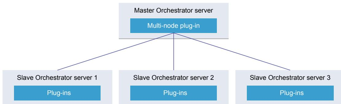
The plug-in contains a set of standard workflows for hierarchical orchestration, management of Orchestrator instances, and scale-out of Orchestrator activities.
