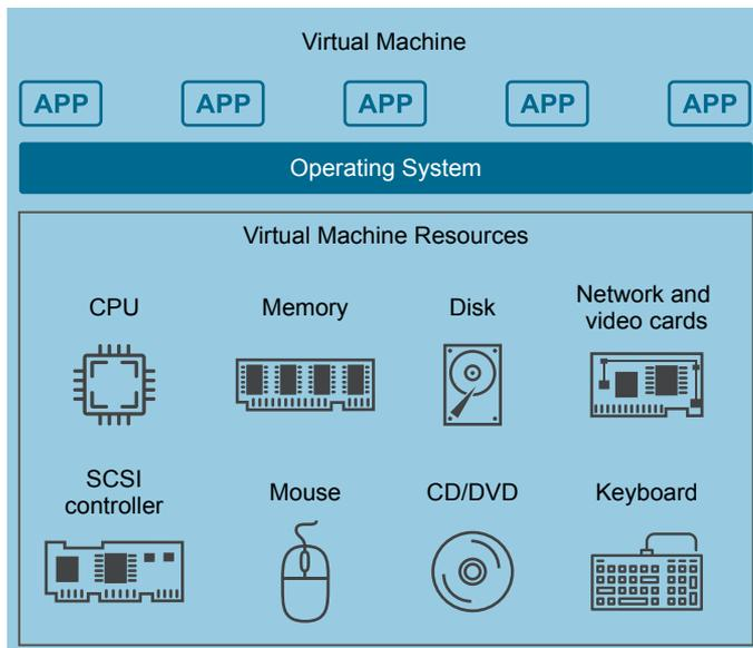
The VMkernel mediates all physical resources. All physical hardware access takes place through the VMkernel and virtual machines cannot circumvent this level of isolation.
